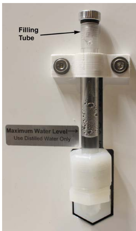
Figure 1: Water Filling Tube
