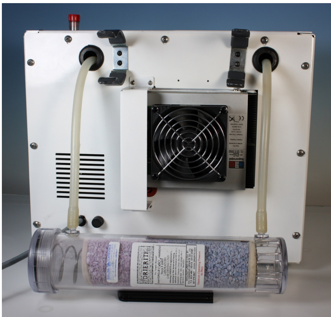
Figure 2: Desiccant Reservoir Pulled From H300P
